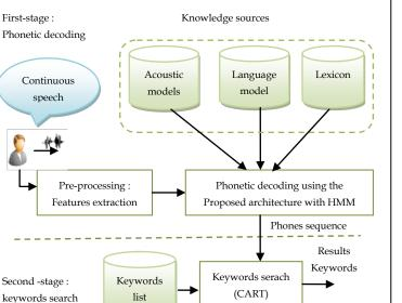
Fig. 1. The two-stage proposed Keywords Spotting system.
